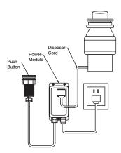
Plug the disposer cord in the power module.
